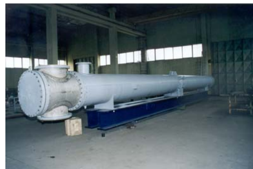
Phosphoric Acid Heater (PFI)
